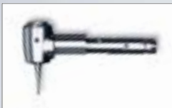
INTRA LUX head 68 LH For removing carious material. To be used with contra-angle handpiece burs. Maximum operating speed: 40,000 min -1 . Features: push-button control, debris deflector and strengthened chuck system. 1:1 direct drive ratio. REF 0.540.2040
